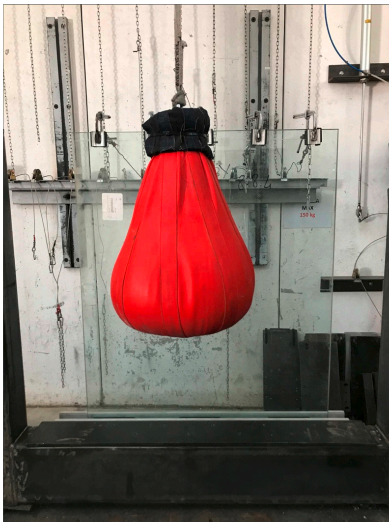
Photograph of the item after impact on the centre of the glazing according to standard NF P01-013:1988
