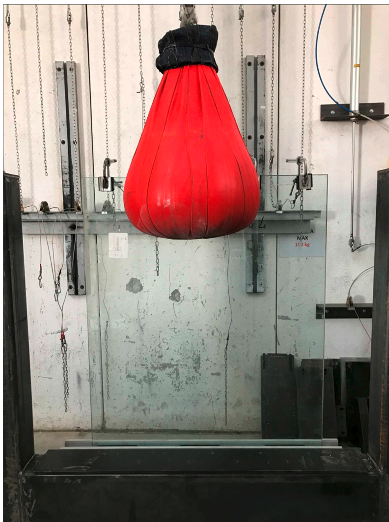
Photograph of the item after impact on the border of the glazing according to standard NF P01-013:1988
